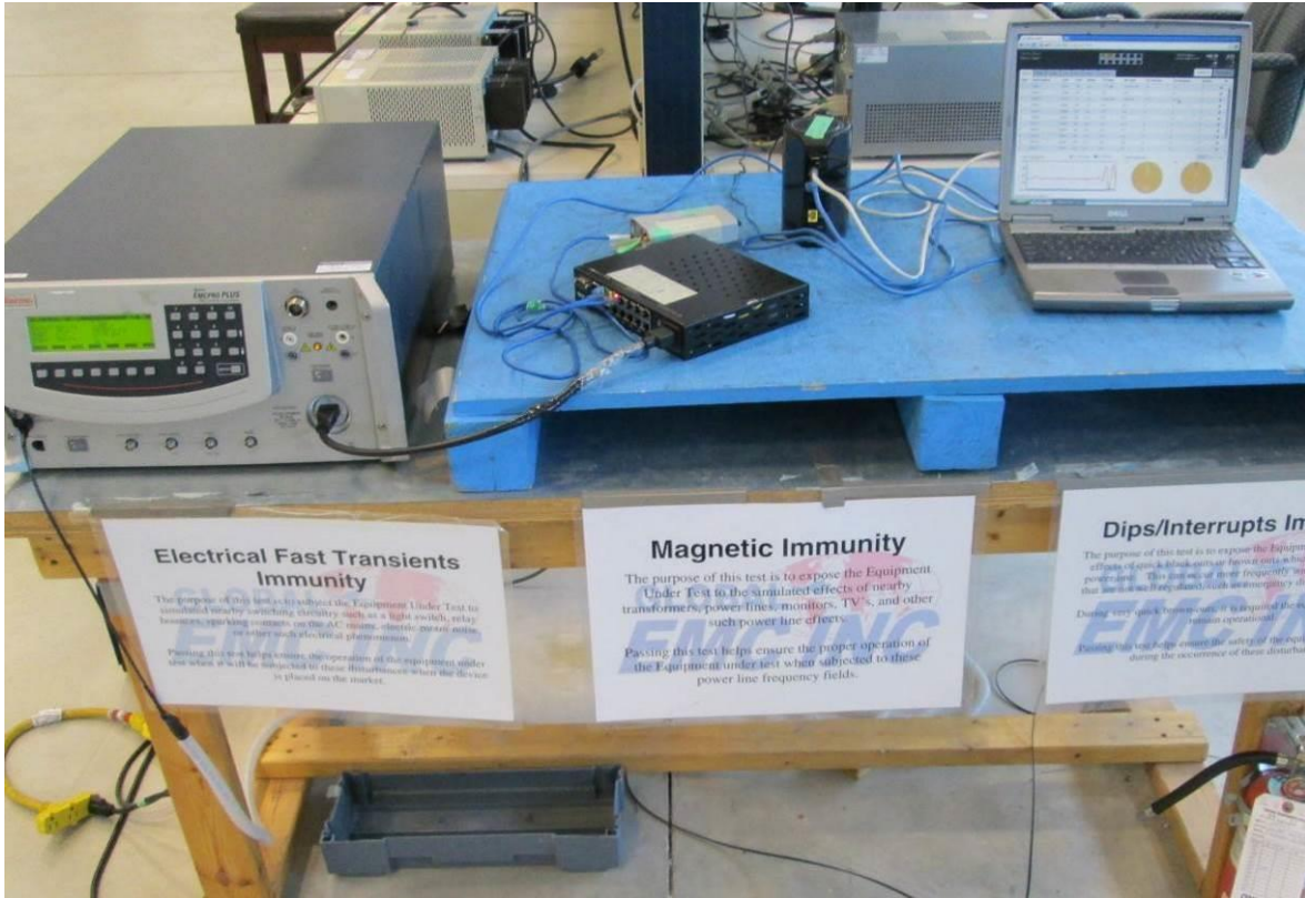
Figure 13 – EFT (AC & DC), Surge (AC only), and Voltage Dips/Interrupts (AC only) Test Setup
