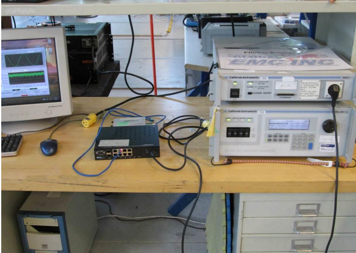
Figure 8 – Harmonics and Flicker Emissions Test Setup
