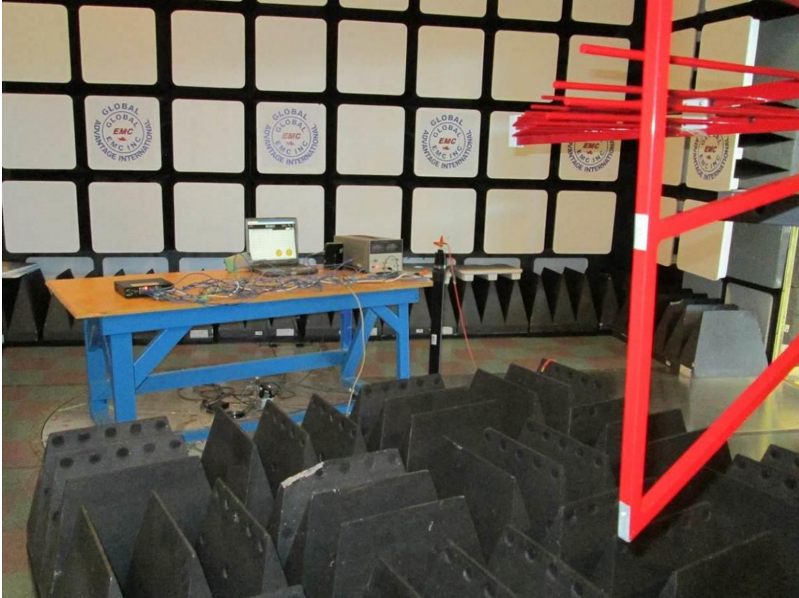
Figure 10 - Radiated Susceptibility Test Setup
